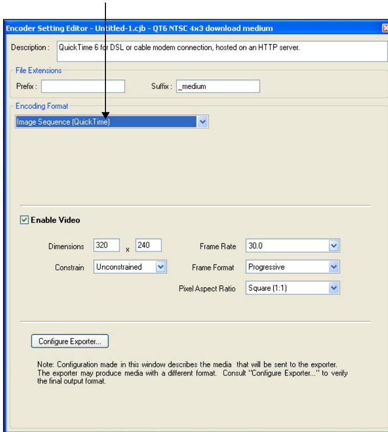
15. Enter the resolution for the exported stills in the Dimensions fields. This should be the same frame size as the input movie file or the TGA files will be distorted.
