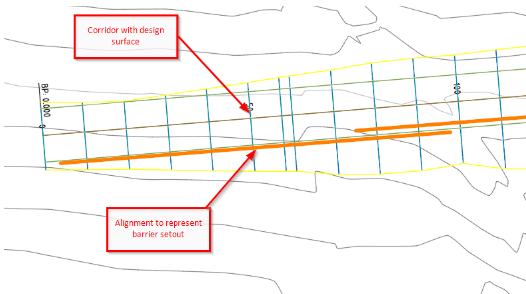
Figure 42: Corridor surface and Alignments
