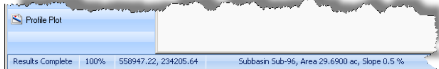
Figure 2.6 The Status Bar provides information about the network model being worked on
