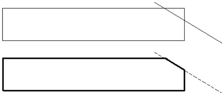
Cut the profile by specifying positions of two points that define a line. Additionally, a direction is indicated (a point on one side of the cutting line): it determines the object part that will be cut.
