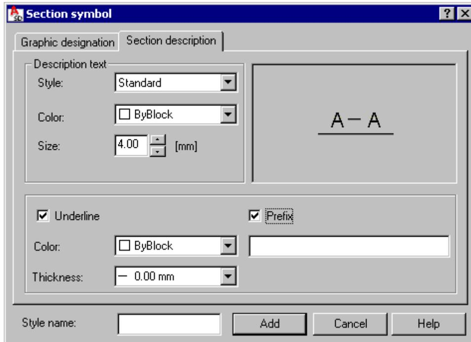
The options located in the *Description text* field specify the description of an RC element section. The following parameters can be set: font style, color and size. Below are two options:
