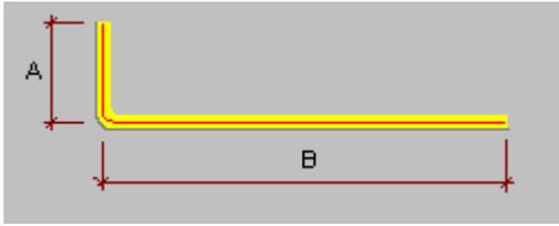
*Total along axis* - if this option is selected, the reinforcing bar length is calculated - in reinforcement tables - as a sum of lengths of segments of the bar with hooks; reinforcement tables specify lengths of bars along their axes.
