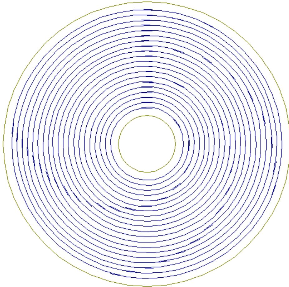
Each bar in the polar distribution is divided separately following the rule: bar of the maximum length + bar of the maximum length + the rest resulting from the remaining length of a bar to be distributed. Division of every bar in the polar distribution starts at the same point.
