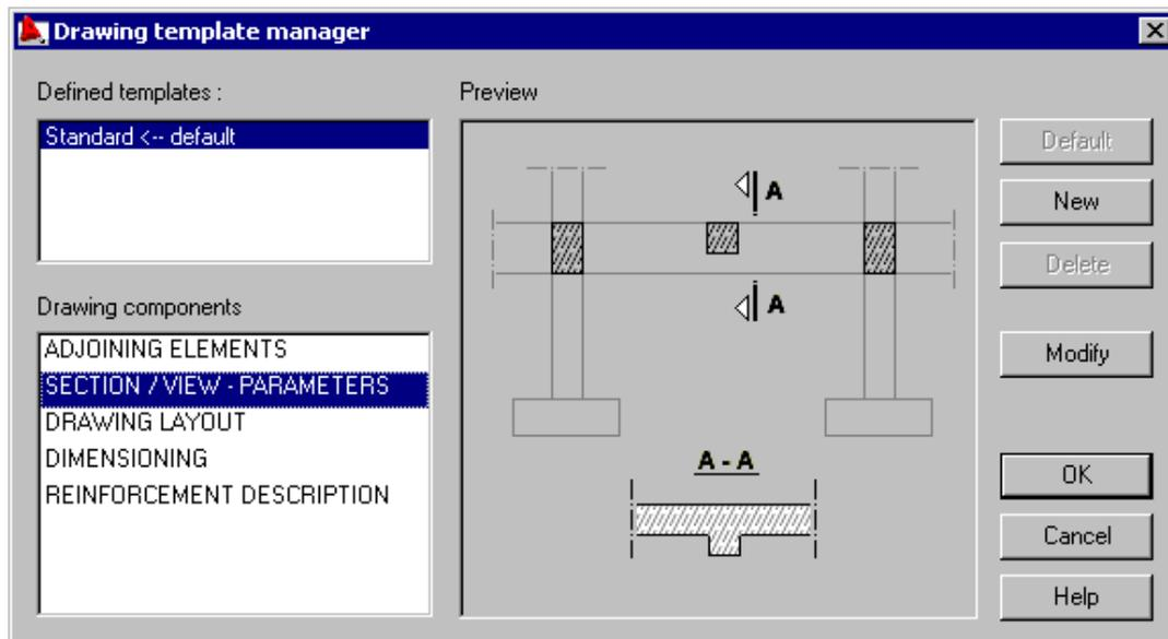
The structure drawings are parametrized by a set of styles. They are divided in groups which parametrize the specified components of a structure drawing of an element.
