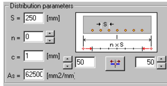
The left side of the dialog contains the parameters controlling reinforcement distribution within one zone:
