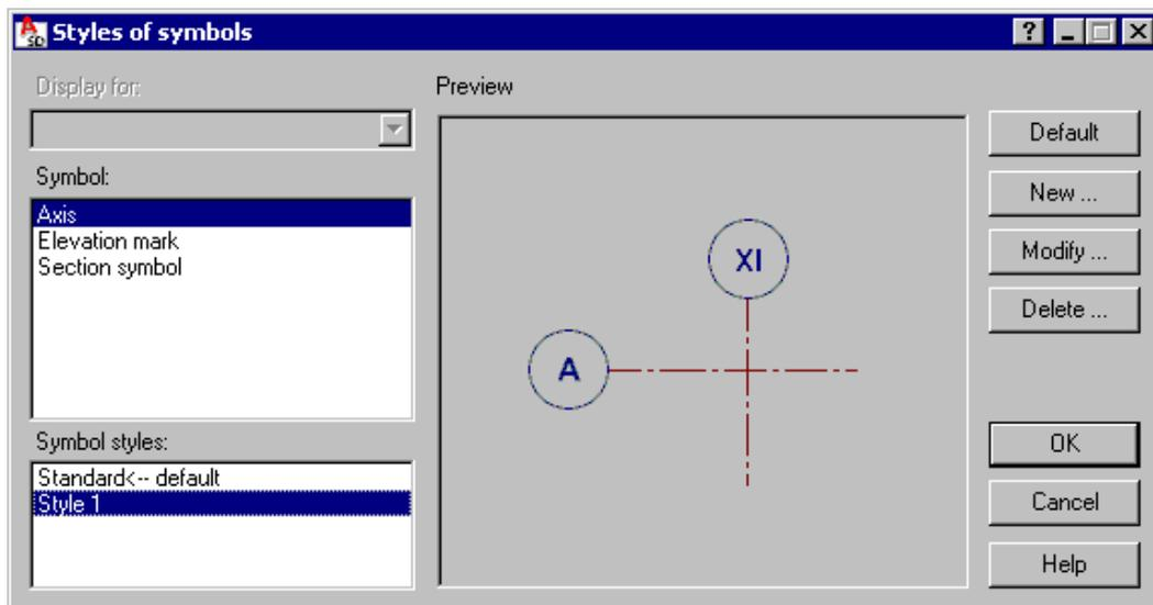
The following types of symbols are used for elements of RC structures (presented in the *Symbol* field in the dialog):
