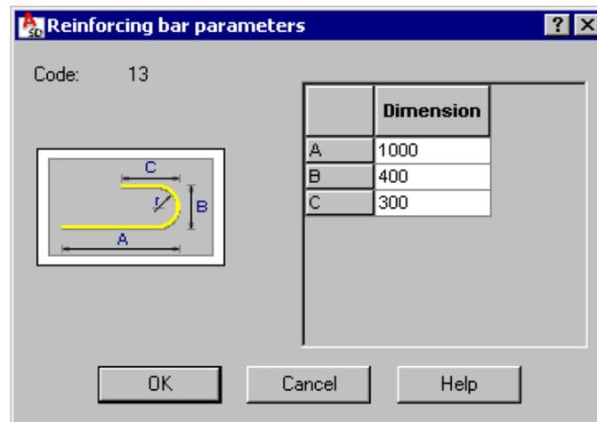
The above dialog contains a table that displays dimensions of bar segments. If the dialog is open while a bar is being defined, then dimensions that are not yet defined are assigned a zero value. You can change the bar segment lengths and to complete the missing dimensions. The field with a shape code is filled out automatically depending on a typical shape selected.
