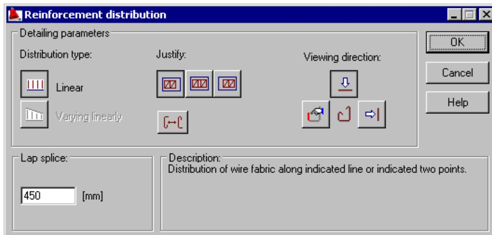
The options in the left side of the dialog, in the *Detailing parameters* field, are used to specify a type of reinforcement distribution:
