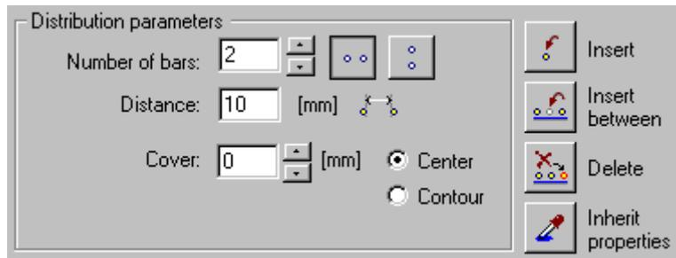
The distribution method is intended for all cases where standard methods of reinforcement distribution prove ineffective. This method allows you to position a bar or a bar group freely, based on the distribution carried out earlier; the distribution may also be defined independently.
