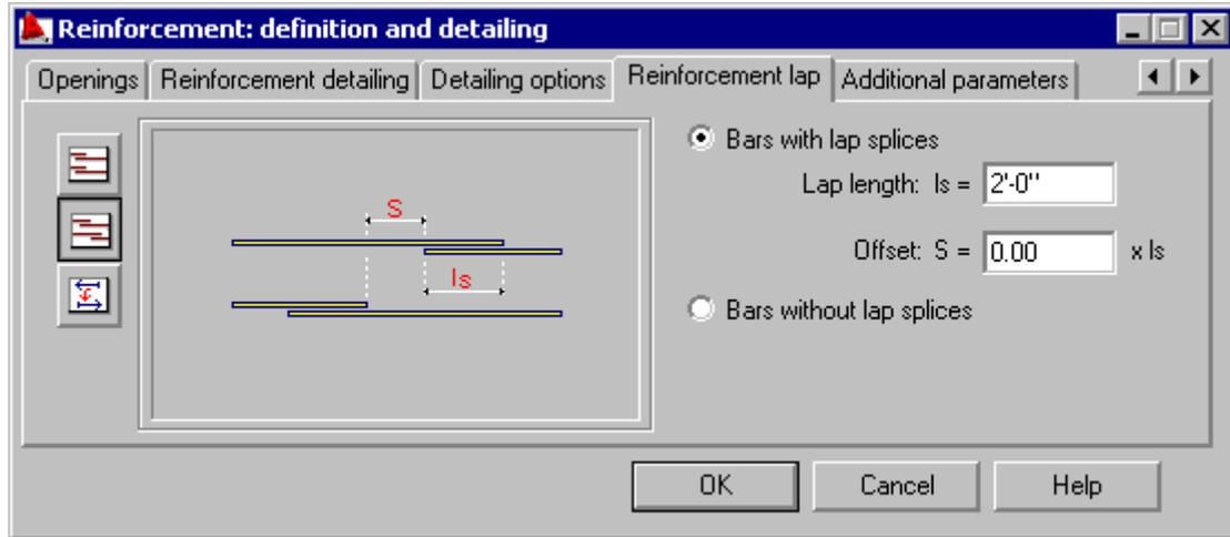
When main reinforcement is being distributed, it may prove necessary to use reinforcement laps. If reinforcement length exceeds the value defined in the preferences (e.g. 12 000 mm), then the options provided on this tab enable defining reinforcement laps (connections of reinforcing bars).
