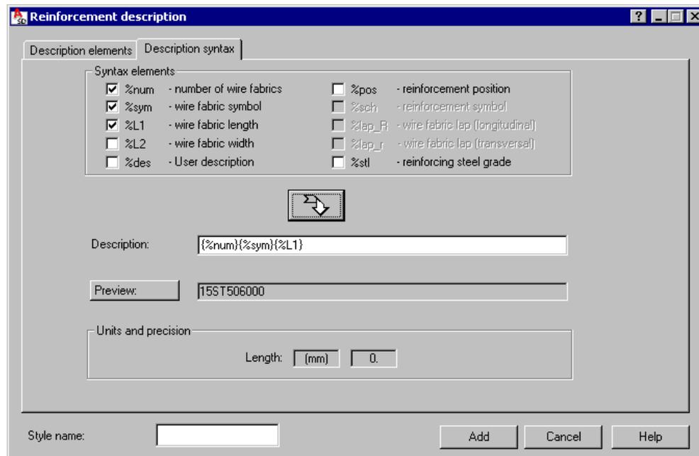
Under Syntax elements, select components and move them to the Description field (by clicking the arrow under the element list), where you can arrange variables with user-defined text and symbols.
