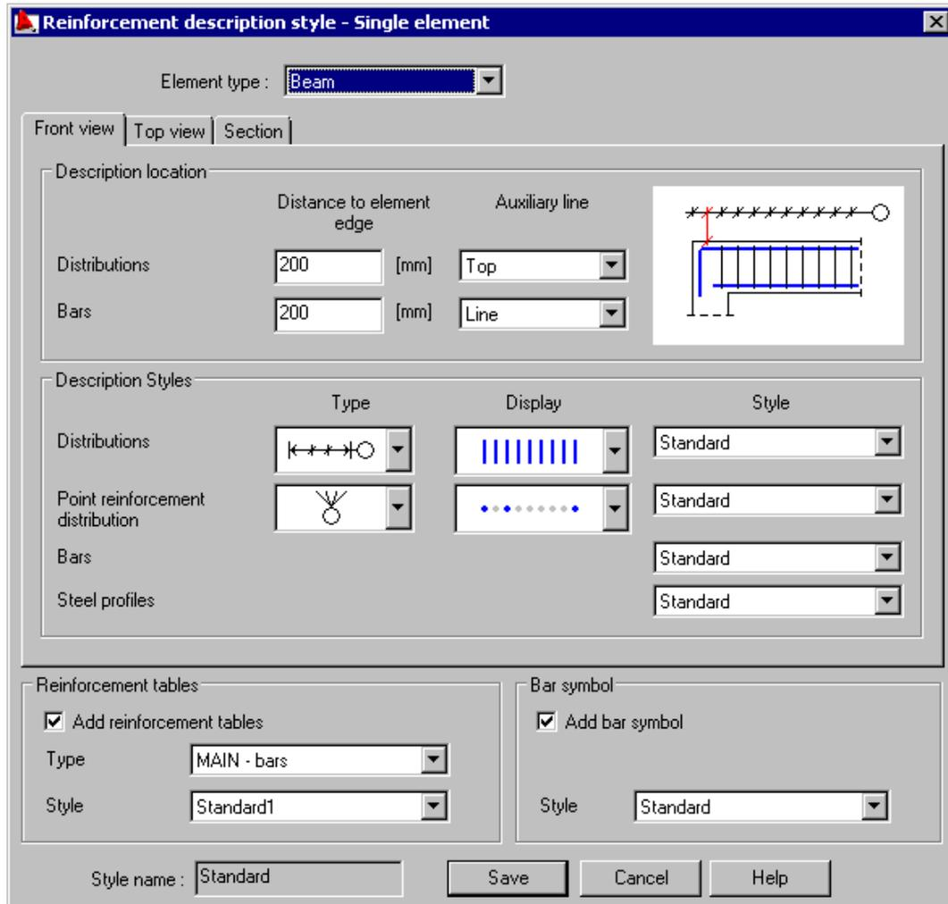
A selection list for selection of a structure element type (beam, column, spread footing, etc.) is located in the upper part of the dialog; it defines for which element the reinforcement description will be defined.
