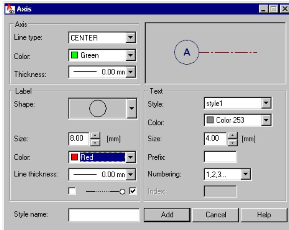
The *Axis* field holds parameters of a line presenting the axis in a drawing: line type, color and thickness.
