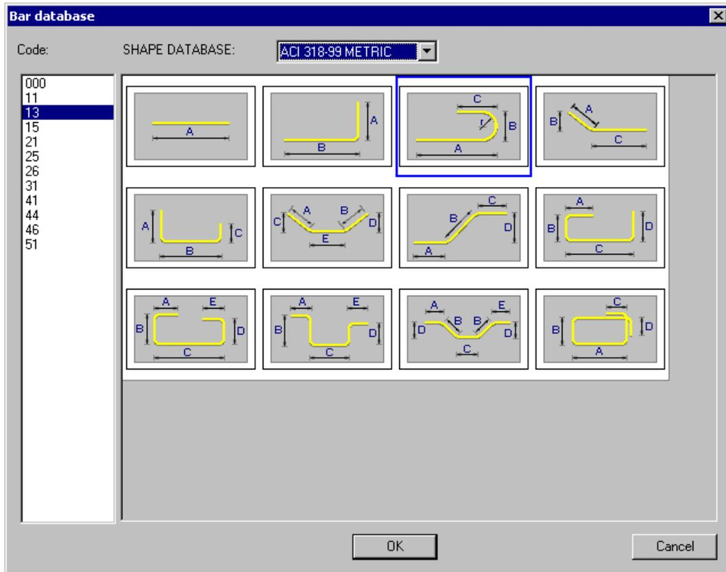
To define bars from the database, select from the available shape list, and define successive bar segments by indicating next bar characteristic points presented in a schematic drawing (you may also enter dimensions of individual segments).
