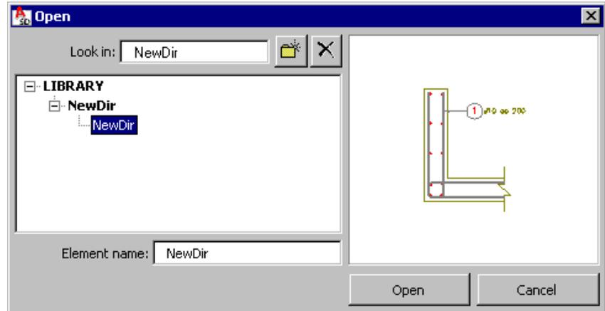
After selecting a saved linear element, a block of drawing elements is placed in a drawing. The linear element chosen is assigned name and length; the spacing of elements over the length (e.g. 3 meters of length with spacing every 20 cm) is also specified.
