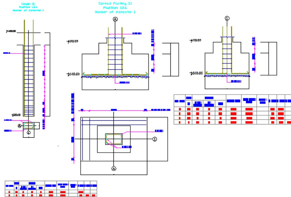
The first stage of drawing generation is to create views in the model space. Create views for projections of the spread footing and the column as follows:
