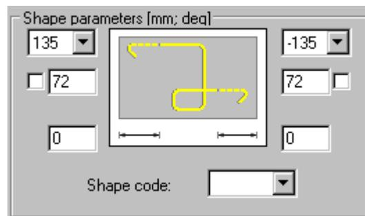
You can select a type of hook at the beginning and end of the defined reinforcement and lock a hook length by selecting the option next to the edit field for defining a hook length ( appears); the edit field becomes inaccessible. If you modify parameters (length or diameter) of a bar with a locked hook length, the hook length does not change.
