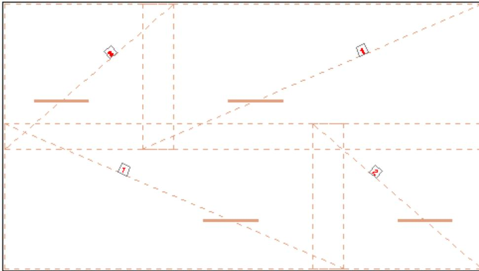
There is also a possibility of simplified presentation of wire fabrics; the drawing below shows the simplified method of presenting a generated wire fabric.
