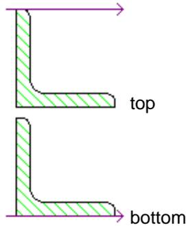
It is also possible to define an offset (shift) of the point of insertion of a steel profile; the offset denotes a shift of the profile center with respect to the insertion axis. An offset value may be positive (offset upwards) or negative (offset downwards)
