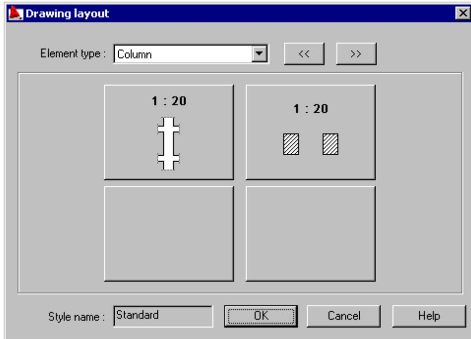
The dialog presents layout of views/plans to which the views or section elements can be assigned.
