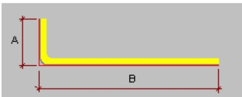
*total* - if this option is chosen, the reinforcing bar length is calculated as the total of lengths of bar segments with hooks; bar lengths are given in compliance with total outer length.
