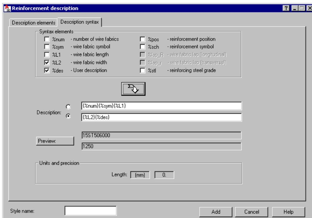
Under Syntax elements, select components and move them to the Description field (by clicking the arrow under the element list), where you can arrange variables with user-defined text and symbols.
