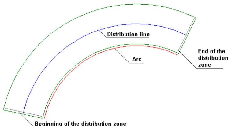
A description of the distribution is an arc-shaped line as for the radial distribution. This line always shows the spacing from the distribution line.
