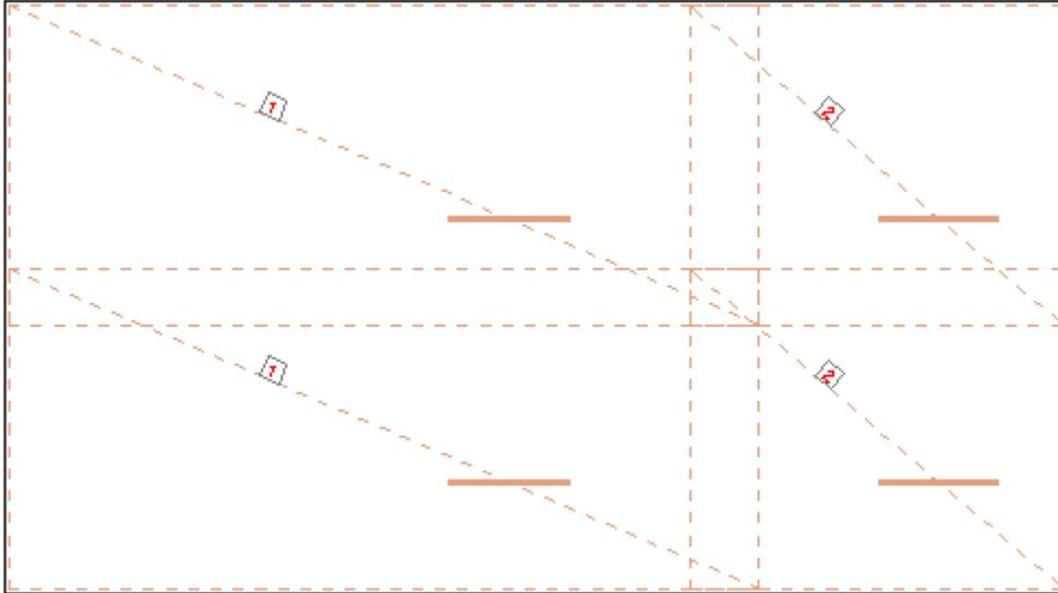
passing and half-way types - wire fabrics are shifted in relation to each other by half the length (to avoid concentration of lap splices of several wire fabrics at the same point) – shown in the drawings below
