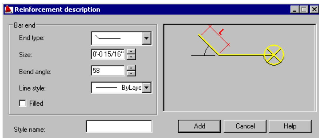
The *Bar end* field has options for presenting reinforcing bar ends (additional lines at bar ends) in distributions. These lines are additional objects connected with the bar.
