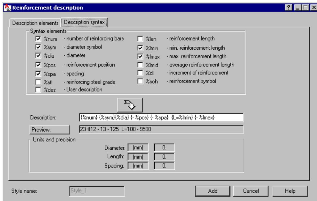
Under Syntax elements, select components and move them to the Description field (by clicking the arrow under the element list), where you can arrange variables with user-defined text and symbols. An example description is: f10 every 15 cm length = 2.0 m.
