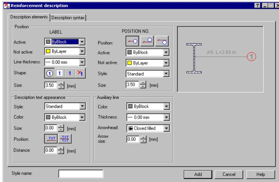
The options in the Position field refer to a label and the number that the label contains (see the drawing below).
