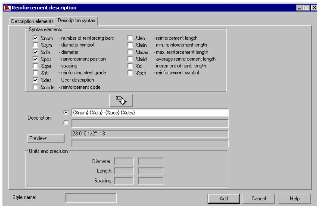
Under Syntax elements, select components and move them to the Description fields (by clicking the arrow under the element list), where you can arrange variables with user-defined text and symbols. An example description is:  $\phi 10$  every 15 cm length = 2.0 m.
