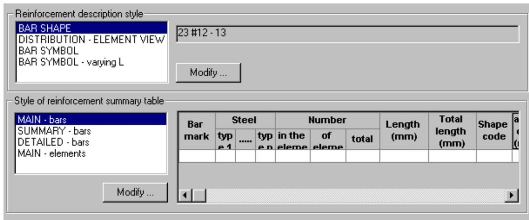
The top part of the dialog includes styles of reinforcement descriptions with reinforcement division into categories considered. Once an appropriate reinforcement category is selected from the list (the category is highlighted), an example description displays based on the settings of the reinforcement description style.
