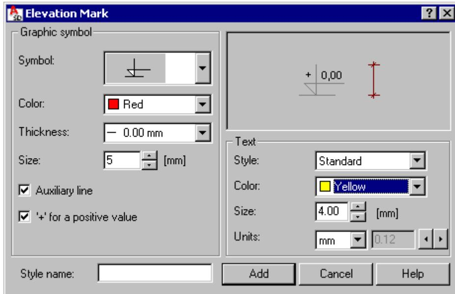
The *Graphic symbol* field holds parameters of a symbol representing a level in the drawing: symbol type, color, size and thickness of the line in the symbol.
