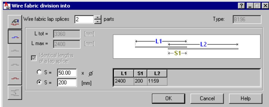
The left part of the dialog contains the following icons used to define the lap splice of a wire fabric:
