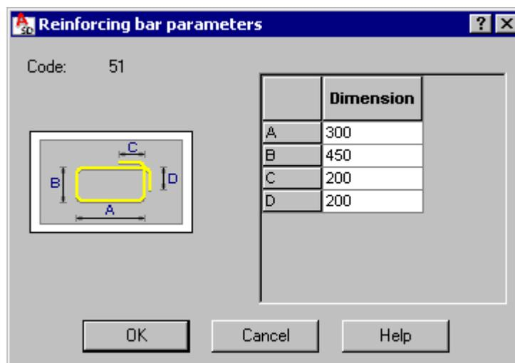
The above dialog contains a table that displays dimensions of bar segments. The field with a shape code is filled out automatically depending on a typical shape selected. Both modes of reinforcement definition are synchronized with each other; both definition modes can be used alternately.
