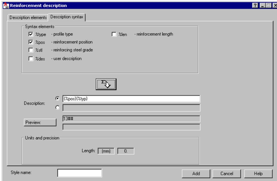
Under Syntax elements, select components and move them to the Description fields (by clicking the arrow under the element list), where you can arrange variables with user-defined text and symbols.
