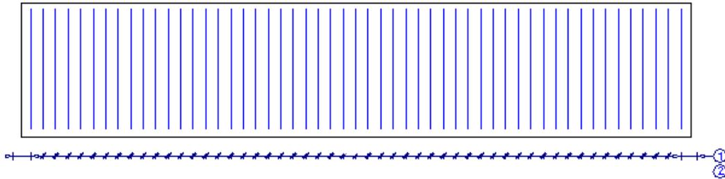
Two bars distributed simultaneously are represented by one line whose length equals the height of the larger stirrup.
