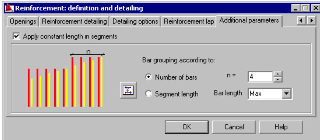
You can select the Apply constant length in segments option in the above dialog. The option allows for automatic bar distribution in case one or more edges is inclined. The option allows to apply so-called constant length in segments, i.e. grouping the bars according to the rule defined in the dialog, and assigning constant length to them in a given group.
