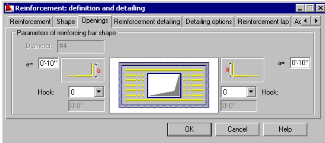
Use this dialog to specify parameters for bar ends near openings. The same end types as for other bars are available for bars that adjoin to openings (see the Shape tab).
