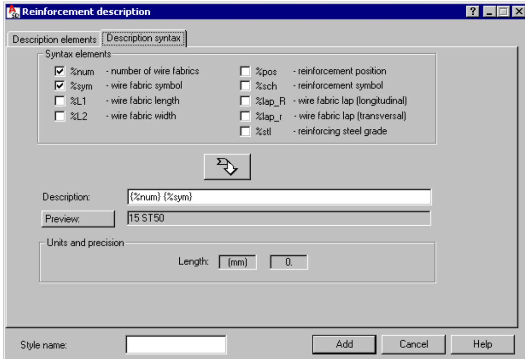
Under Syntax elements, select components and move them to the Description field (by clicking the arrow under the element list), where you can arrange variables with user-defined text and symbols.
