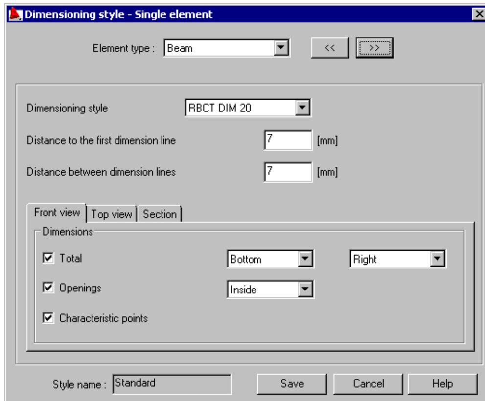
A selection list for selection of a structure element type (beam, column, spread footing, etc.) is located in the upper part of the dialog; it defines for which element the dimensioning parameters will be defined.
