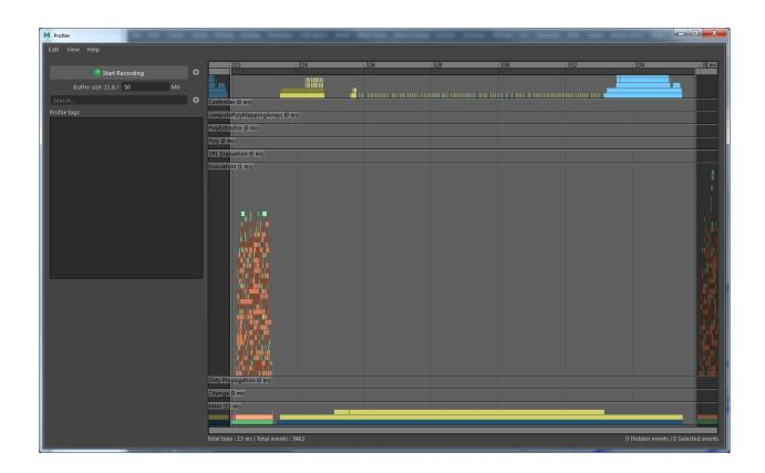
In the second image the footPrintNode\_GeometryOverride has been modified to support Evaluation Manager Parallel Update. You can see that the long serial execution time in Vp2BuildRenderLists has been eliminated. All the data marshalling for VP2 is occurring in parallel while the Evaluation Manager is evaluating the Dependency Graph.
