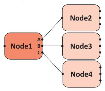
In this graph, evaluation first calculates outputs for Node1 (that is, Node1.A, Node1.B, Node1.C), followed by parallel evaluation of Nodes 2, 3, and 4 (that is, Read Node1.A to use in Node2, Read Node1.B to use in Node3, and so on).
