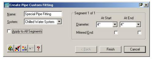
Need a unique fitting? Try creating an intelligent one using simple AutoCAD entities.
