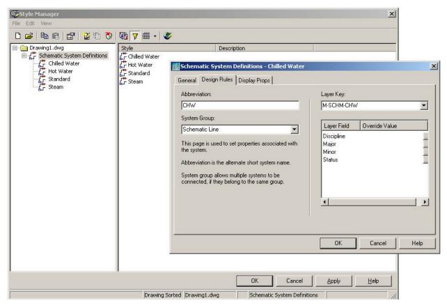
Assign schematic system definitions for easier management of detail properties.
