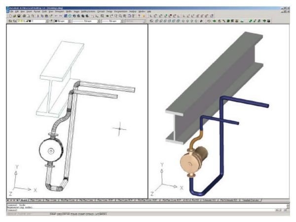
Get to pumps and other mechanical equipment in hard-to-reach places using flexible pipe.
