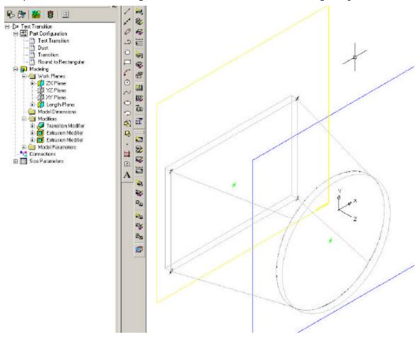
Use the Content Builder to produce parametric MvParts and fittings.
