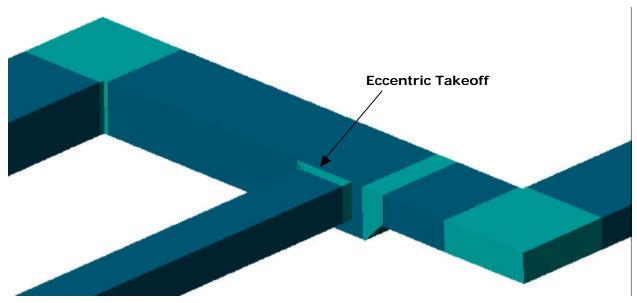
When space is at a premium, every inch counts. Route your ductwork and piping adjacent a chase wall or to the underside of structural beams.
