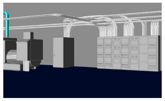
Use interference detection with electrical MvParts in tight electrical rooms.
