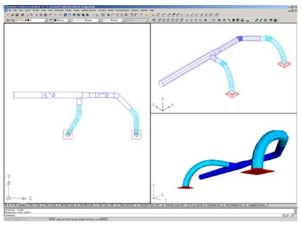
Use flexible duct to connect to your diffusers and grilles or show a flexible connection to equipment where vibrations might be a concern.
