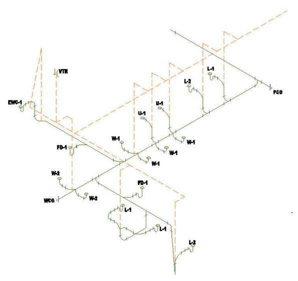
Produce isometric riser diagrams quickly and easily.
