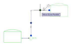
2 Click the stretch grip in the middle of the top horizontal line, and move the line up slightly. Click the new location to place the line.
