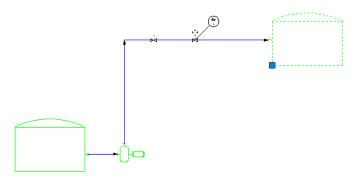
2 On the bottom-left corner of the selected tank, click the grip and drag the tank to the left, about half the length of the horizontal line. Click again to place the tank in the new position.
