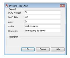
**Note** Make sure you add the drawing number to all drawings in your project. You can then track drawing-specific data in the Data Manager, which displays the drawing number for all components and lines that are part of this drawing. The drawing number is particularly important when you are using an off-page connector to continue a line from one drawing to another.
