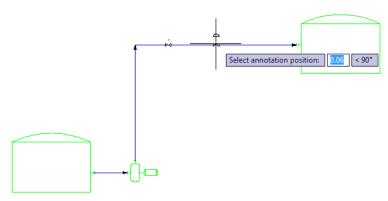
A leader line is automatically placed to connect the annotation bubble to the control valve.
