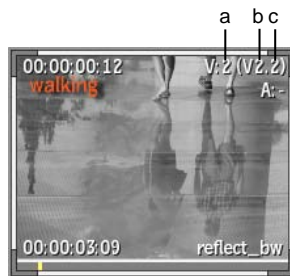
(a) Total number of video tracks (b) Focus is on track V2 (c) Focus of track V2 is on topmost layer, L2
