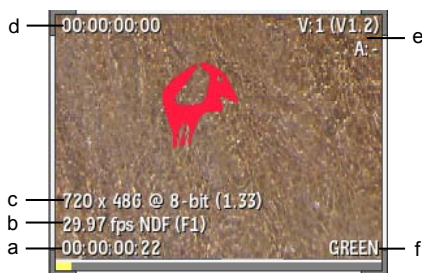
(a) Clip duration (b) Framerate and Scan mode (c) Resolution, bit depth, and aspect ratio (d) Current timecode (e) Track information (f) Clip name
