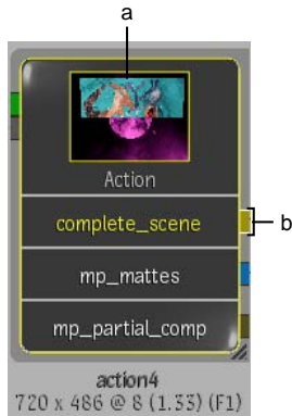
(a) Proxy of complete_scene output (b) Yellow text indicates proxy of output is displayed
