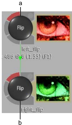
(a) Flip node connected to left eye is edited (b) Settings are automatically duplicated on Flip node connected to right eye
