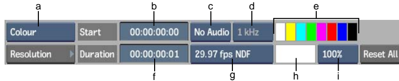
(a) Source Type box (b) Start field (c) Track box (d) Frequency box (e) Colour palettes (f) Duration field (g) Frame Code Mode box (h) Source colour pot (i) Luminance box
