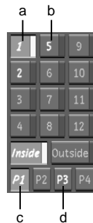
(a) Selected and activated secondary layer (b) Activated and unselected secondary layer (c) Current secondary layer page with activated layer(s) (d) Secondary layer page with activated layer(s)
