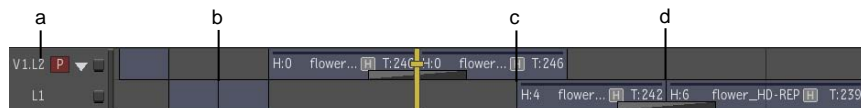
(a) Focus layer (L2) (b) Cut on L1 seen through gap of focus layer (c) Cut on L1 not seen through focus layer (d) Transition on L1 seen through gap of focus layer
