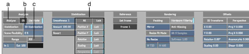
(a) Analyze button (b) Stabilization Method box (c) Region of Interest button (d) Stabilization Parameter buttons
