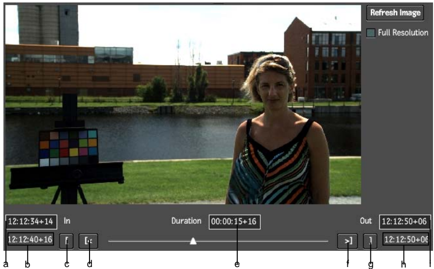
(a) In timecode (b) Start timecode (c) Mark In button (d) Go To In button (e) In-Out duration field (f) Mark Out button (g) Go To Out button (h) End timecode (i) Out timecode
