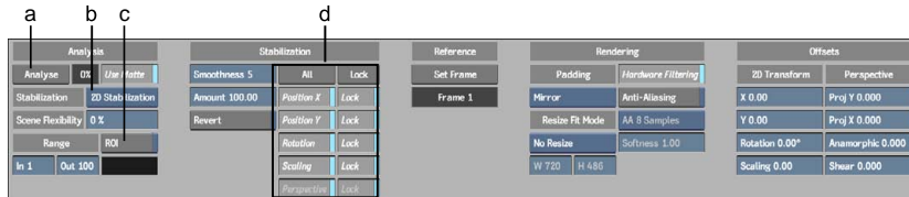
(a) Analyze button (b) Stabilization Method box (c) Region of Interest button (d) Stabilization Parameter buttons
