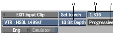
(a) Bit Depth box (b) Aspect Ratio field (c) Scan Mode box
