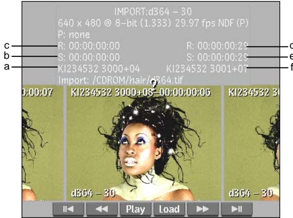
(a) Start keycode for the clip (b) Start Source Timecode for the clip (c) Start Record Timecode for the clip (d) End Record Timecode for the clip (e) End Source Timecode for the clip (f) End keycode for the clip
