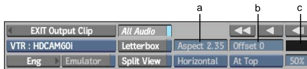
(b) Letterbox aspect ratio field (c) Letterbox offset field (a) Colour selector box
