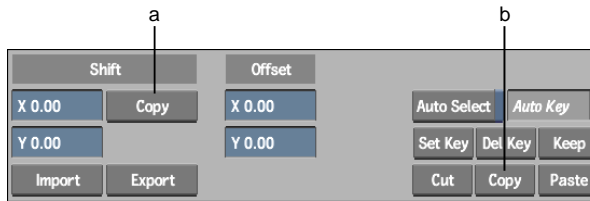
(a) This Copy button takes the aspect ratio into account (b) This Copy button does not take the aspect ratio into account
