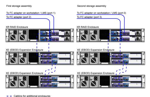
NOTE In a configuration with two XR RAID enclosures, the number of XE extension enclosures per XR RAID enclosure must be the same. The total number of enclosures in the storage assembly must be an even number.
