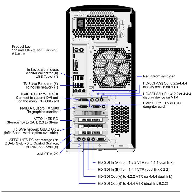
NOTE This diagram depicts a Gigabit Ethernet (GigE) adapter located in PCI slot five. Your workstation may also be configured with an optional QuickSilver InfiniSERV 9000 PCIe-DDR adapter. On the HP xw8600 workstation, the PCI slots are numbered one to seven from top to bottom.
