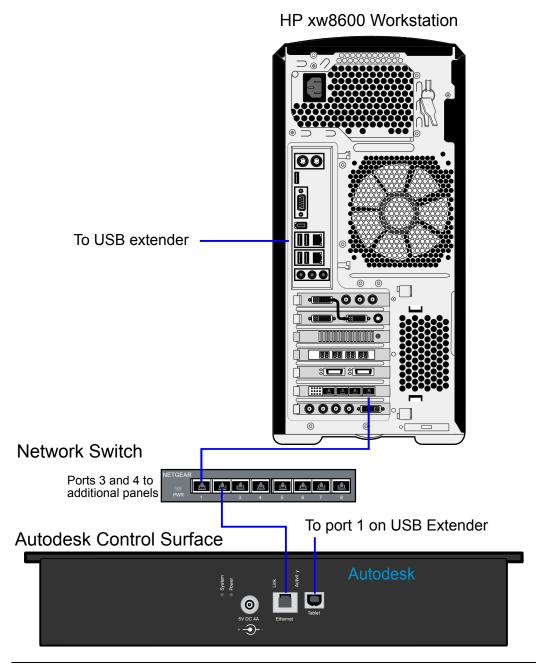
NOTE The illustration shows the central panel only (the Colour Grading panel). This panel is easily identified, since it has both an Ethernet network port and a USB connector. It is also the panel with the built-in tablet.
