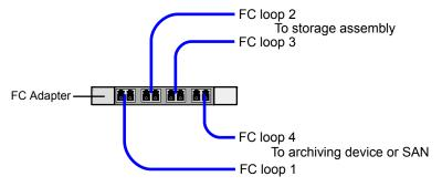
NOTE If you are not using all the ports of a fibre channel adapter, terminate the two unused ports with the FC loopback couplers that shipped with your system. Terminating these ports significantly decreases the time required to boot the system.
