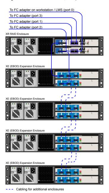
NOTE In a 4-loop configuration with a XR 6412 RAID enclosure, you need a minimum of one XE expansion enclosure attached to the XR RAID enclosure.
