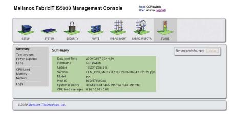
**3** Click Ports in the menu at the top. The Ports page appears, displaying an overview of the switch. Connected ports are displayed in green.
