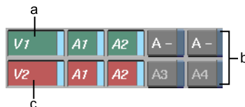
(a) Source Primary video track (b) Patch boxes (c) Record Primary video track
