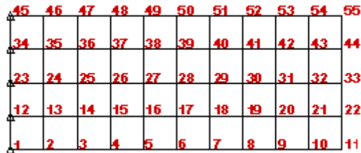
Figure 2-2: Square Elements in Example "skewuss"
