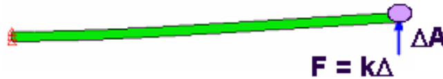
Figure 166-4. Diagram of the deflection at point A in the beam due to the spring load.
