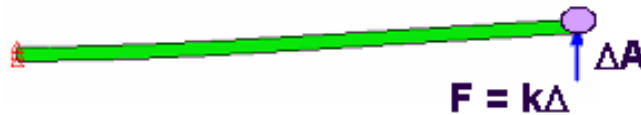
Figure 156-4. Diagram of the deflection at point A in the beam due to the spring load.
