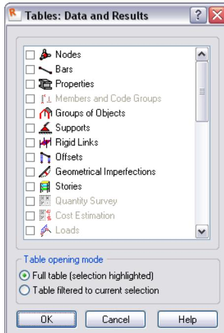
In this dialog box, one should indicate the required items and press the **OK** button. A table containing data will be generated for each of the indicated items. Once the *Edit* tab is activated in the bottom left corner of a given table, one may perform the operation of modifying structure parameters.
