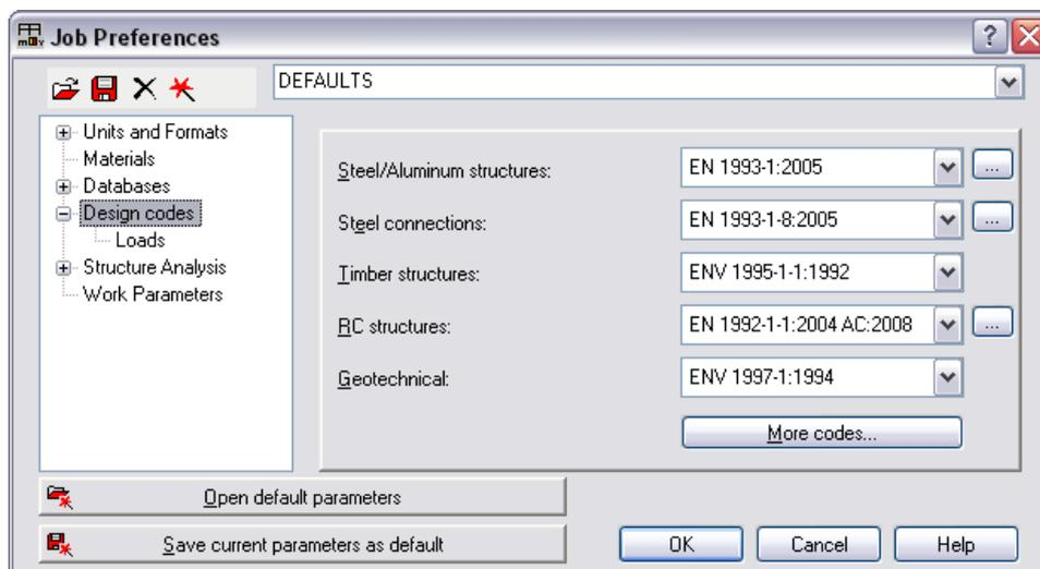
**Job Preferences** are grouped in six categories: units, materials, databases, design codes, structure analysis and work parameters.
