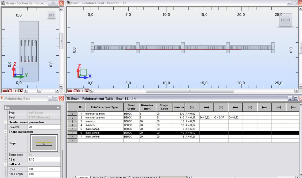
The screenshot displays the reinforcement design process for a beam. It includes a cross-section view, a longitudinal view, a 'Reinforcing Bars' dialog box, and a 'Reinforcement Table'.
