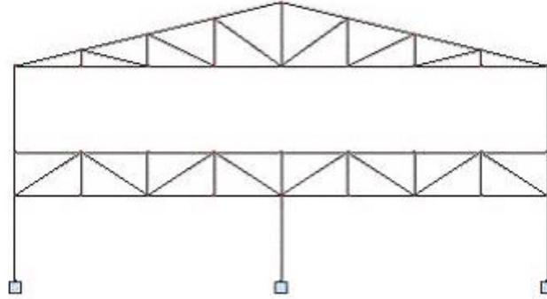
Three load cases will be applied to the structure (self-weight and two load cases: wind and snow, shown in the figure below). Moreover, a moving load case will be applied to the structure.
