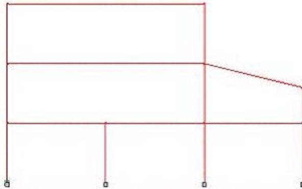
Three load cases will be applied to the structure (self-weight and two cases of live loads presented in the drawing below). Moreover, (10) load cases generated automatically for snow/wind loads will be applied to the structure.
