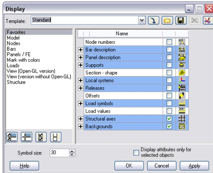
The available tabs allow one to get access to the data on structure parameters. This option is also available from the main menu by means of selecting the *View menu / Display* command.
