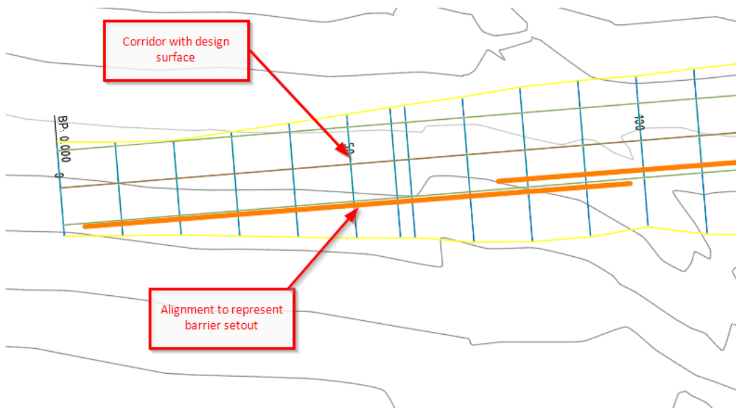
Figure 42: Corridor surface and Alignments
