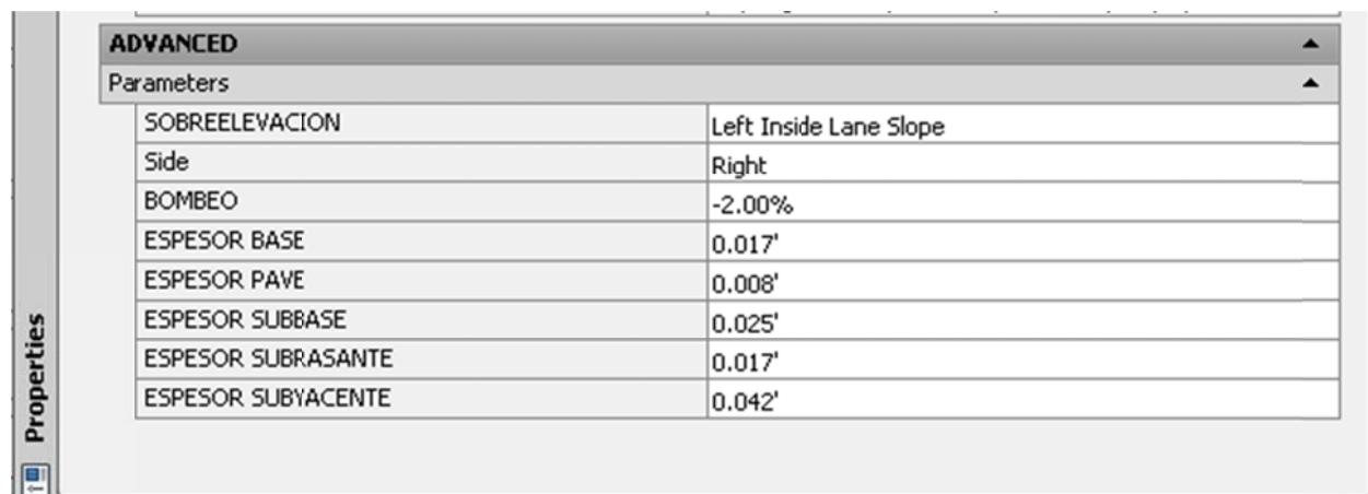
**HOMB\_5\_CAPAS\_Cu\_AFIN A NIVEL DE SUBRASANTE (Shoulder\_5\_component SUBGRADE LEVEL insertion point)**
