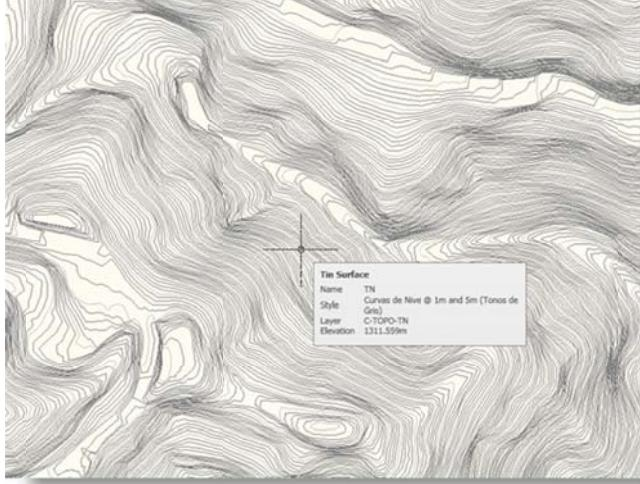
A screenshot of an AutoCAD interface displaying a dense network of surface contours. The contours are rendered in various shades of gray, creating a topographic map effect. A small callout box in the bottom right corner provides details about the surface: <p>Top Surface<br/>Name: TN<br/>Style: Curvas de Nivel @ 1m and 5m (Tonos de Gris)<br/>Layer: CTOPO-TN<br/>Elevation: 1311.559m</p> |         |
