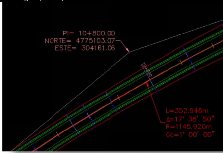
A screenshot of AutoCAD showing a road alignment with geometric labels. The labels include:<br>PI= 10+800.00<br>NORTE= 4775103.07<br>ESTE= 304161.06<br>L=352.946m<br>$\Delta=17^\circ 38' 50''$<br>R=1145.920m<br>$O_c=1' 00' 00''$ |         |
