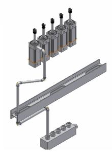
The custom tube and pipe style is applied to the pipe route. It uses at least one pipe and one 90-degree elbow that you published into the Content Center library.
