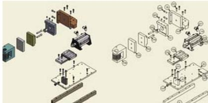
With drawing views you can quickly create assembly drawings and exploded assembly views for use in training manuals and manufacturing instructions. With the Autodesk Inventor presentation environment you can easily create compelling animated sequences for use in training videos, assembly instructions, and sales presentations, helping you visually communicate your design intent.
