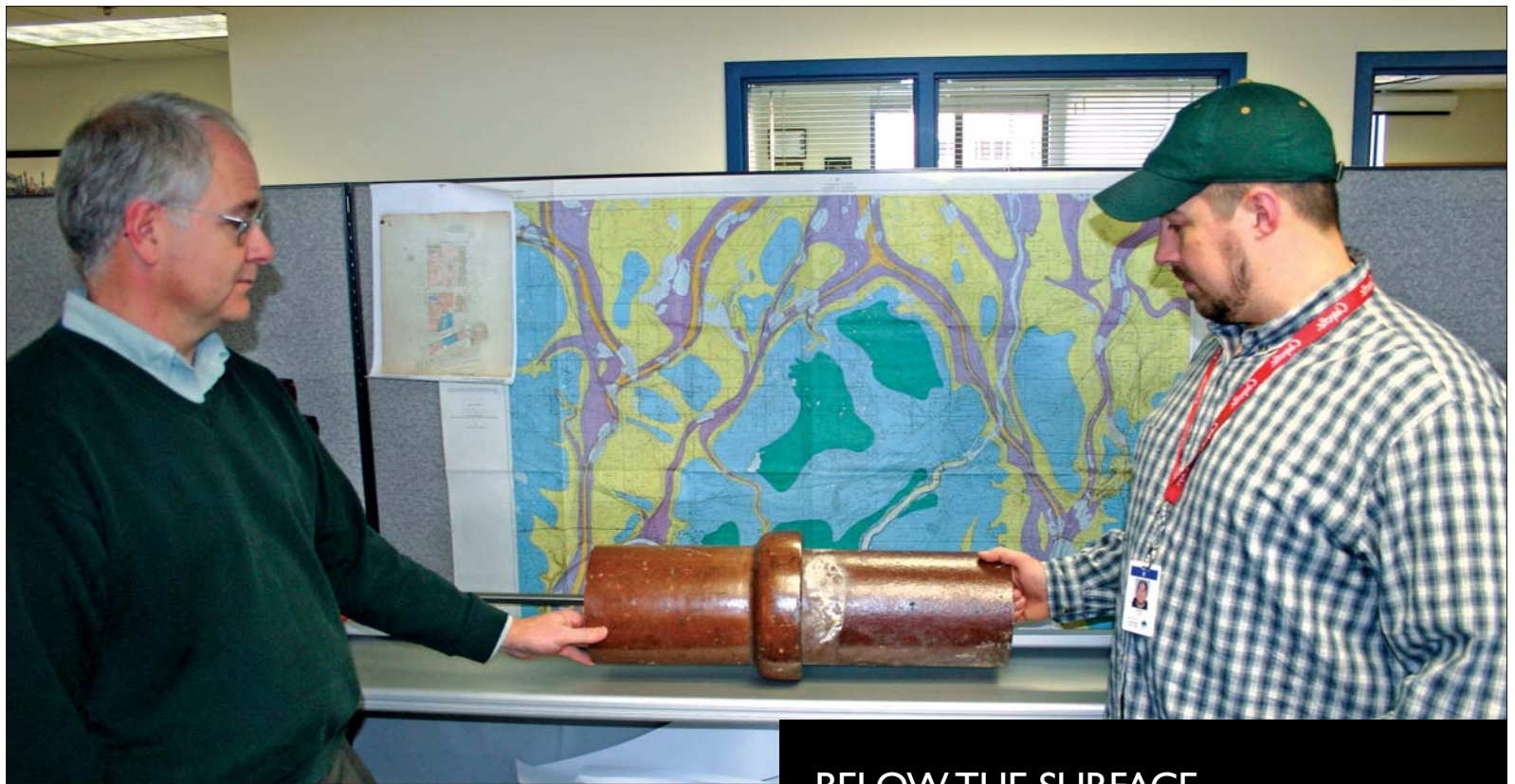
Engineering aide technician Paul Ackerly (right) and civil engineer Dan Bartholic display a section of vitrified clay pipe, the most common type used in St. Paul. All types of pipe are shown on the city's new digital maps that replaced 2,500 paper maps.
