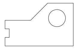
2 Offset the lines to create walls (if it's a health spa or motor housing) or ridges (if it's a catch for a window lock). Use a value for the offset distance that is appropriate for what you are creating. Clean up the corners using Fillet with the fillet radius set to 0.
