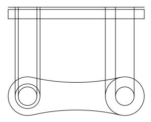
7 Trim the four vertical lines representing the silhouette edges of the holes as shown. Don't forget to press ENTER after selecting the horizontal boundary line for the trimming.
