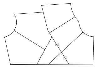
**14** Draw a short property line using the endpoint object snap between the end points of the property lines as shown.
