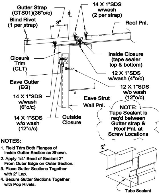
Gutter Splice Assembly
