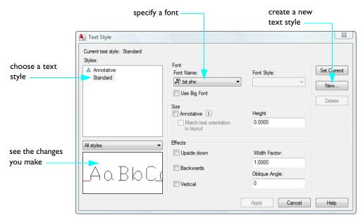
If you change an existing style's font, all text in the drawing that uses that style is regenerated using the new font.
