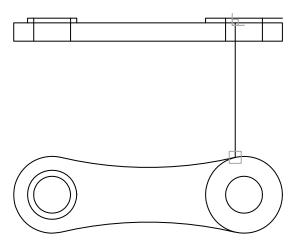
**II** Trim the horizontal line to the boundary line as shown.
