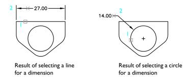
Use object snaps to specify the extension line origins, and then specify the dimension line location. The extension line origin points can be on separate objects.
