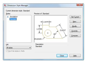
*Overrides* allow for style modifications to the current dimension style. Overrides apply to all subsequent dimensions created with that style until you make a new style current. They do not permanently modify a dimension style. You can also override properties of dimensions using the Properties palette.
