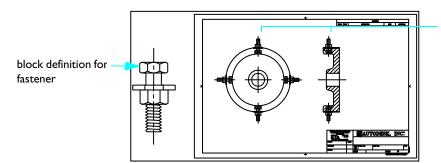
block references of fastener inserted into a drawing
