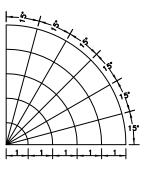
The polar tracking feature displays visual guidelines at specific angles and can snap the cursor to an angle.
