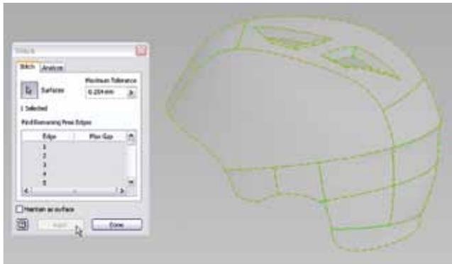
At this point in the design, the surfaces can now be used with many of the Inventor features. For example, you could change/add to the part thickness with the “Thicken/Offset” feature found in the Modeling section of the ribbon bar.
